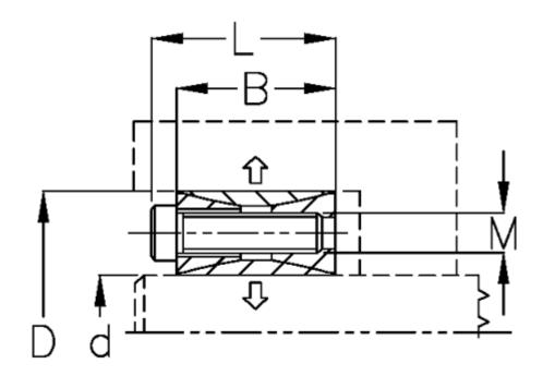
$\begin{array}{lll} \text{B mm} & = 28 \\ \text{d H8 mm} & = 85 \\ \text{D mm} & = 125 \\ \text{Fit tolerance} & = \text{Aksel k11-h11, Nav N11-H11} \\ \text{F kN torque} & = 95.2 \\ \text{L mm} & = 38 \\ \text{M mm} & = \text{M10} \\ \text{P N/mm2 surface pressure on shaft/hub} = 52 \\ \end{array}$
